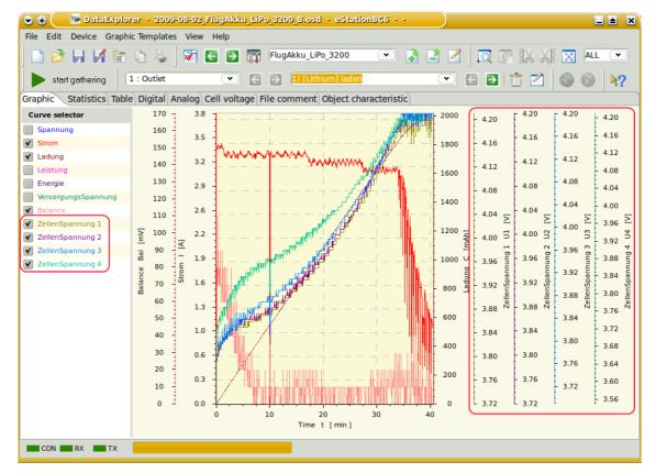
This will make more room for the curve display itself and the minimum and maximum values are the same. Through this the curves are easy comparable and a manual adjustment using the context menu is obsolete.
