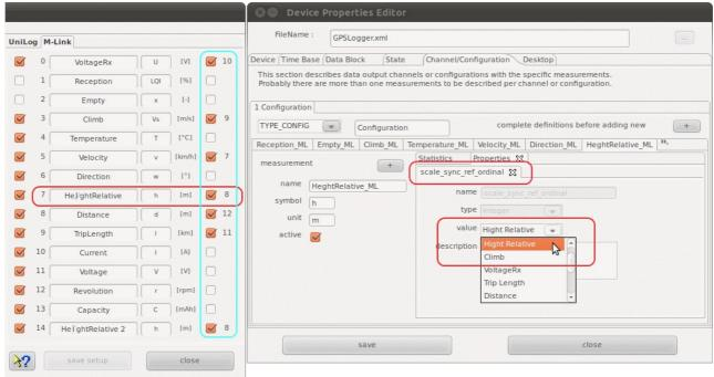
At the right hand side of the configuration panel are check boxes which enable a semi automatic scale synchronization. While checking measurement name will be compared to previous once and the fitting measurement ordinal will be added to the measurement configuration entry. Using scale synchronization will reduce the required space for scales and spend more for the graphics. Overlaying curves in this matter will allow direct comparison without using the curve compare window.
