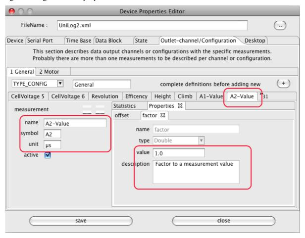
If Multiplex sensors are connected, the units are overtaken from the log data as well. The names and symbols must be manually adapted. The initial presets are only samples. Multiplex M-Link sensor measurements has always a trailing 'ML'.
