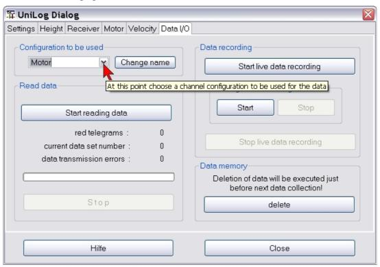
After pushing "Start reading data" all the data within the device are going to be red and the read operation starts immediately and the selected configuration is applied.
