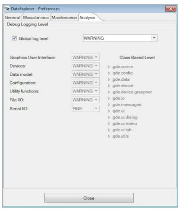
The class based log level allows to set a logging level for selected class(es) which reduce the amount of trace statements and helps analyzing class centric. A context menu enables the log level
