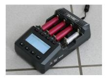
The MC3000 is providing two device descriptions. A MC3000-Set is storing all collected data sets in a single file. It makes sense to choose continuous record set in settings. This will help to keep track of the slot to data set relation. In such a case four simultaneously processed batteries will result in one record set per battery and all four record sets will be stored in a single file.
