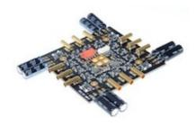
The device represents a specialized solution used as driver for quadro copters and monitor its usage data. The log files following CSV notation and can be imported for visualization. The log data contains driver data as well as batterie data for exact evaluation.
