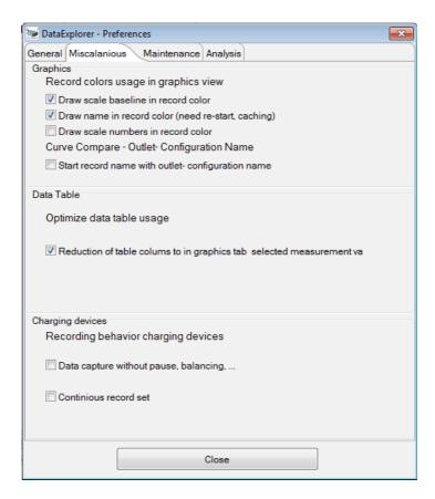
The data table consist of a lot of columns. It is possible to reduce the visible columns to the measurement values selected in the graphics view. This can be adjusted using the context menu of the data table as well.
