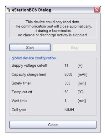
Afterwards the serial communication port adjustments are done using the device selection dialog the start button can be used to initiate data collection.
