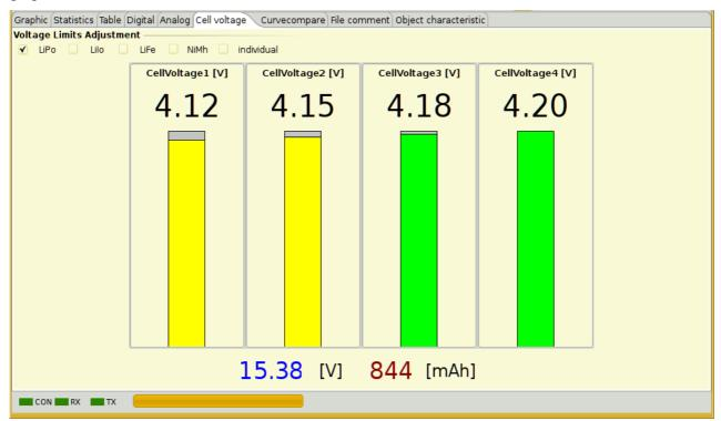
If the voltage values of the displayed cells has only a small difference the bar graph will spread to make differences more visible. If a cell voltage is lower than 2.60 Volt or above 4.20 Volt the bar color will change to red. If the cell voltage is between 2.60 and 4.20 Volts the bar is colored yellow. The bar color changes to green if the cell voltage is exact 4.20 Volt.
