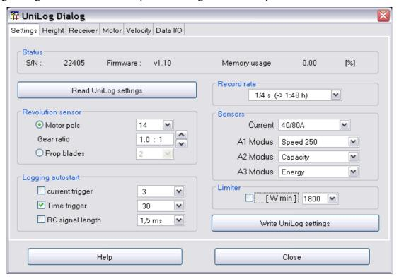
All analog outlets are to be pre-configured starting with firmware 1.10. By activating the limiter function the signal to the motor controller are reduced reaching the adjusted consumed energy. To
