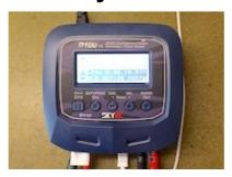
The D100 is a charger with two different independent outlets. With the actual available firmware the previous measured internal resistance will not get transport into the data gathered as it is stated in the manual. A future firmware will possible update this behavior.
