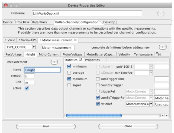
In addition a proportionality gets calculated to show the used battery capacity versus the height during motor runtime. This allows judgments how effective the available power is used up.
