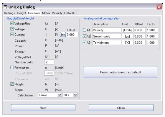
If the measurement "Height" will be selected the dependent measurement slope calculation with its two combo boxes gets activated.
