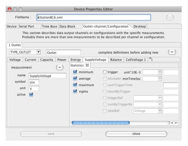
Underneath the area where the type and the name has to be configured another tabulator describes the individual measurements. The measurement configuration is responsible how the data are finally displayed in the various windows including the unit and the statistic mathematics.
