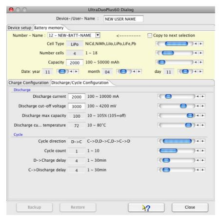
**Hint:** Only parameters gets displayed for configuration purpose which has a relevance for the selected cell type. The configuration of step charge parameters are actually not possible and is part of future release.
