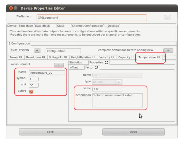
If Multiplex sensors are connected, the units are overtaken from the NMEA data as well. The names and symbols must be manually adapted. The initial presets are only samples. Multiplex M-Link sensor measurements has always a trailing 'ML'.
