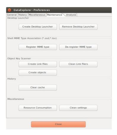
The button "Create Link Files" will scan all data files under the configured folder and create all missing object directories as well as the associating link files. The button "Clean Link File" will delete object related link files but not the object description files nor the object related directories. This function helps to move data files to different system/platform or for backup purpose.
