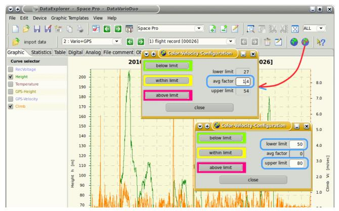
The dialog is displayed twice to make the velocity configuration behavior more clear (blue circled). Is an average factor set to zero, the minimum and maximum velocity fields can be used to configure different values. While the average factor is not equals zero the minimum and maximum values gets calculated.
