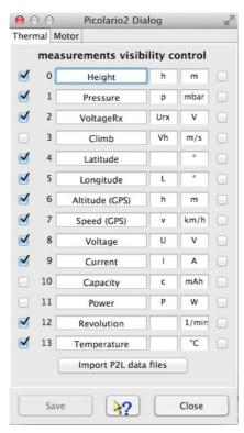
At the right hand side of the configuration panel are check boxes which enable a semi automatic scale synchronization. While checking measurement name will be compared to previous once and the fitting measurement ordinal will be added to the measurement configuration entry. Using scale synchronization will reduce the required space for scales and spend more for the graphics. Overlaying curves in this matter will allow direct comparison without using the curve compare window.
