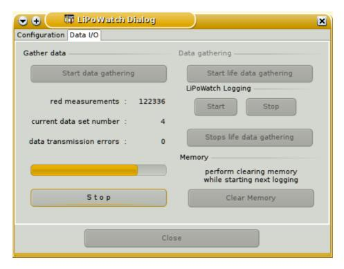
At the end of the read operation the data are displayed. The dialog gets back to its initial state. Only the progress bar is filled and the number of red measurements are displayed.
