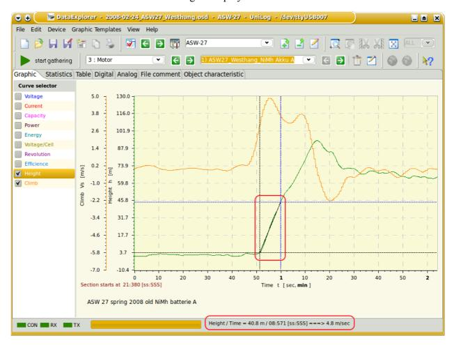
As measurement hairlines black and blue hairlines are displayed. Adjust both as described before to measure a single curve point value. Especially in zoomed curved this makes sense. As additional information the starting point of the zoomed area is displayed.
