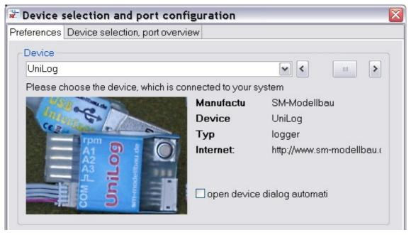
The selection of the active device can be done in several places on this tab. First place is the combo box direct above the device picture or with the slider at right hand side of the combo. The picture of the just selected device will be shown. Additional information related to the device is shown at the right hand side of the picture. Direct underneath this device info two selections are available to configure device specific behavior regarding device dialog and communication port.
