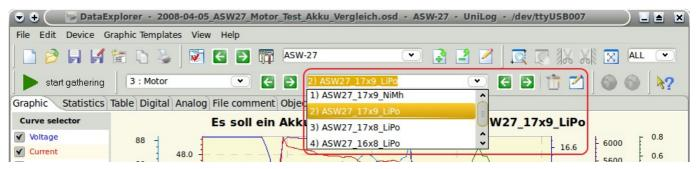
At the right hand side there are buttons to enable data set name editing or deletion. After pushing the edit button the cursor within the data set name field is activated for editing, a hit to enter commits this operations.
