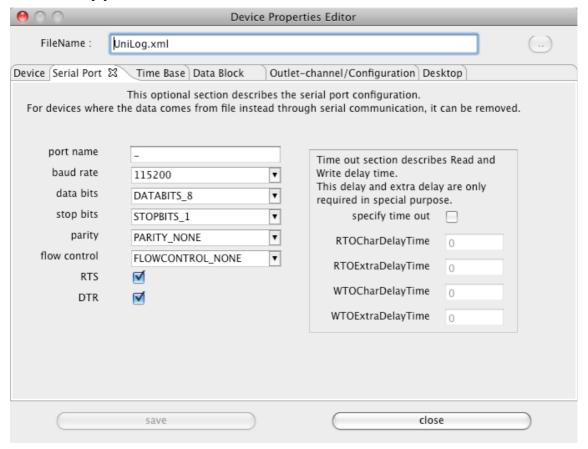
The serial port gets configured easily by selecting appropriate values from the combo boxes.
