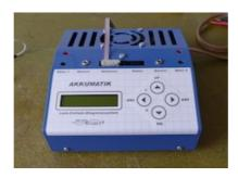
A high quality charging device which is also available as a do it yourself kit. The device supporting reading of data only, it is not possible to store a charge program from outside.
