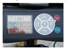
The 4D-Akkumonitor is used to collect data from big battery packs with multiple cells while racing sports. Data gets imported as comma separated files. This files contains beside the cell voltages loop counts and times and GPS data.
