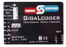
A powerful logger based an Multiplex-Serial-BUS sensors an, writing log data to SD-card. Connect this SD-card using an adapter to your PC to import the log data files for evaluation.
