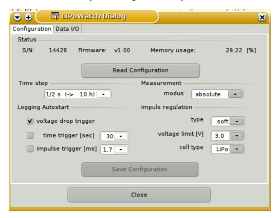
If configuration settings are modified the button "Save Configuration" gets activated. Pushing this buttons will write the modified settings data into the LiPoWatch device.
