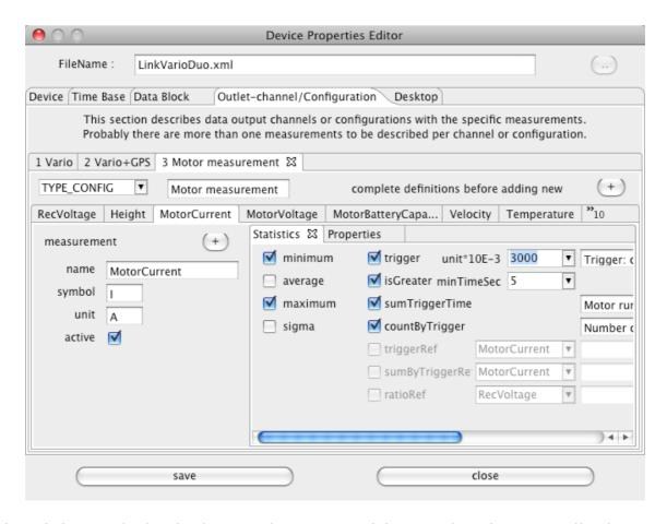
This statistics sample showing how to select average minimum and maximum as well as how to configure a trigger. A trigger is described by a value and a time to be specified as a limit. All average, minimum, maximum and deviation are related to this trigger now. In addition it is shown how to configure that the time where the trigger is active gets summarized. This might calculate the real motor runtime. It is also possible to count the trigger events.
