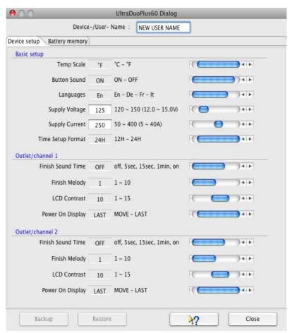
If the serial communication port is selected using the device selection dialog, the port will be automatically opened while opening the dialog and some configuration data will be gathered from the device. To select the battery memories the drop down gets used. The adjustment of the parameter values can be done by using the slider on right hand side or when value field has white background by typing.
