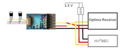
**Hint:** If a HV2BEC is configured and connected the external temperature changes to HV2BEC temperature, external temperature 2 to external temperature 1 .... external temperature 5 to external temperature 4!
