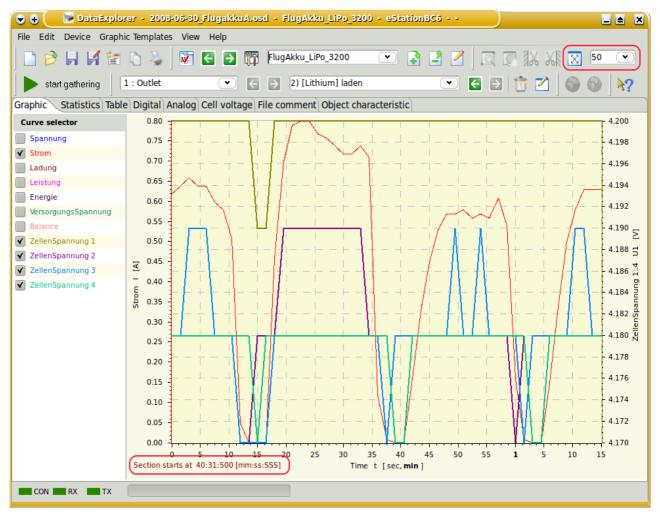
At the menu tool bar the pull down is marked up which just show a selection of the last 50 measurement points to be displayed. Below the time scale the time value of the masking time frame will be displayed. This gives an overview about the total time consummation of the measurement. The sample showing four balanced voltage curves of Lithium cells.
