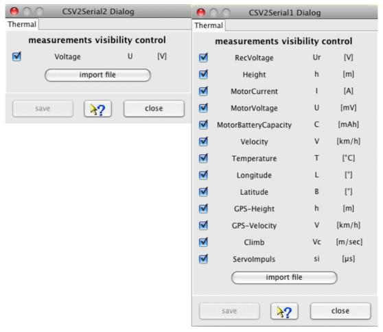
**Hint:** The configured visualization profile is also used if a channel/configuration is selected using the tools bar combo box and the data are imported with the "import file" button.
