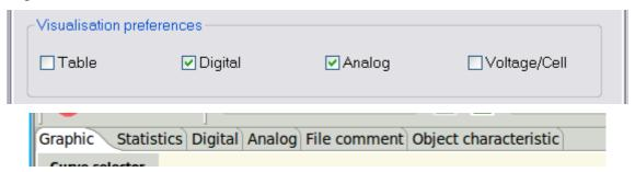
The check boxes in the middle, Digital and Analog, are used mainly for live data measurements and have less sense for devices without this capability. If a device does not have live data capability or data are red from file the end values of the curve are displayed. The visualization of single cell voltages makes only sense for device with the capability to show this, mainly Lithium battery charger or balancer.
