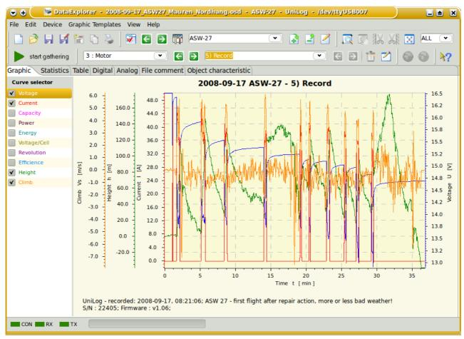
At the bottom there is a status bar to display serial communication status, like connected, receiving and transmitting. Aside the communication port status a progress bar is placed to show progress of long therm operations. The rest of this status area is used to display warning messages or measurement results.
