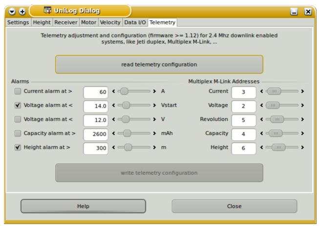
While a configuration will be changed, the button to write the updated configuration into the UniLog, will be enabled.
