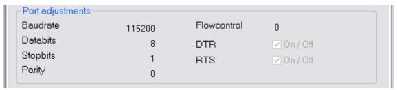
At the lower area the serial communication parameters are displayed without the possibility to change it. Required changes can only be done by editing the device properties XML directly.
