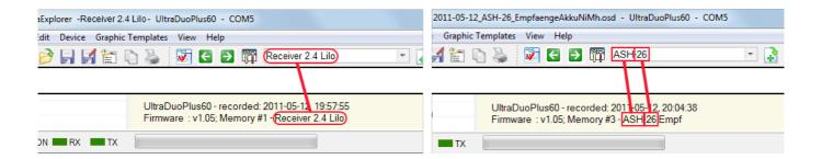
**Hint:** To have good matching results, name battery memories as well as object key names accordingly. Both names battery memory name as well as object key name can be renamed if required
