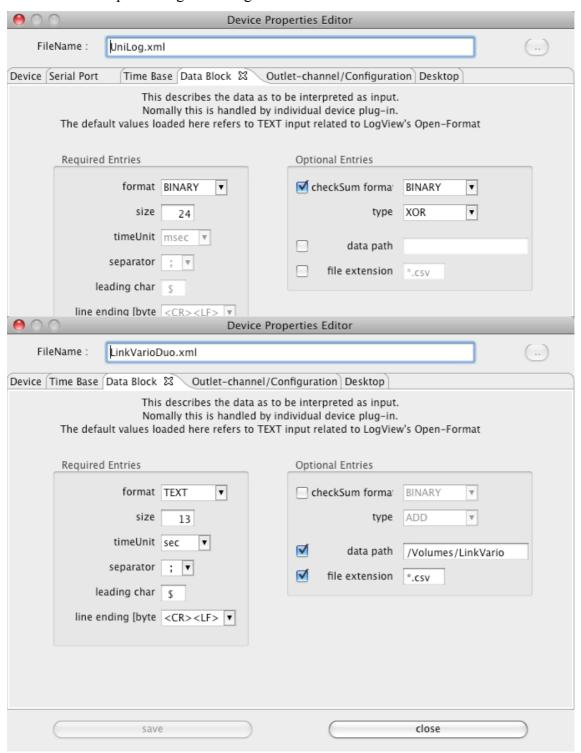
Is TEXT chosen as data type additionally configuration parameter must be specified. The file extension, what is used during file selection, as well as the standard data path, will help to select files faster. Both are optional, but help, if data files are delivered by a memory card, like the DataVario from WStech, which will appear with a dedicated path value if inserted into the computer.
