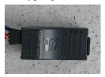
The S32 is the successor of the legendary Jlog2.\*, but internally there is a dramatically change. The S32 is a multi talent regarding connectivity and extensibility. Using an extension up to 16 cell voltages can be monitored. To configure the S32 you need a micro USB cable and a Windows PC. Due to the complexity of the configuration, comparable to an expert system including firmware update, this program will not be ported to different operating systems.
