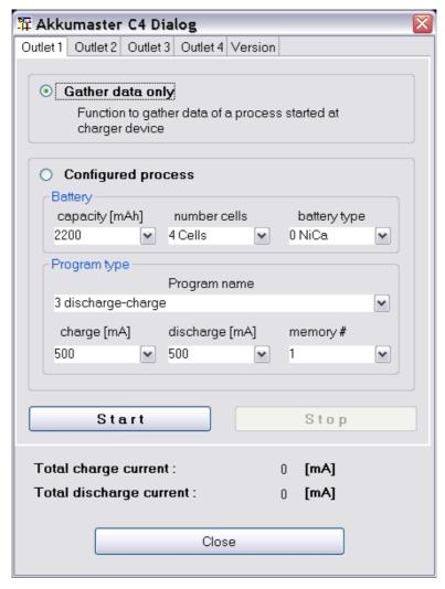
After the start button is pushed all the graphics displays are updated by the gathering cycle. The stop button gets activated to enable stopping of the process for some cases. New data sets get created while the device switch between charge and discharge. The gathering process stops automatically if the device signals no activity anymore.
