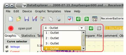
The data set to be displayed can be selected be the other combo box. Analog to the outlet channel/configuration there are buttons to switch to previous or next data set if applicable.
