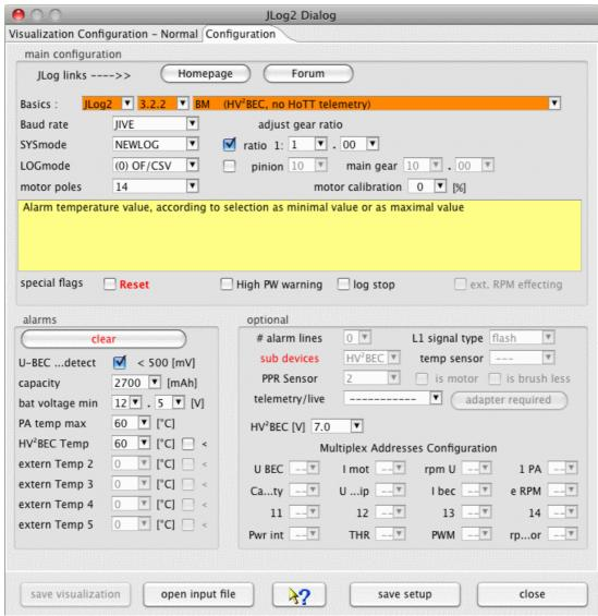
After changing some configuration values saving changes will be enabled. The CONFIG.txt file should be written to identical location as red before. Afterward the SD card can be removed from the system and inserted into the slot of the JLog2.
