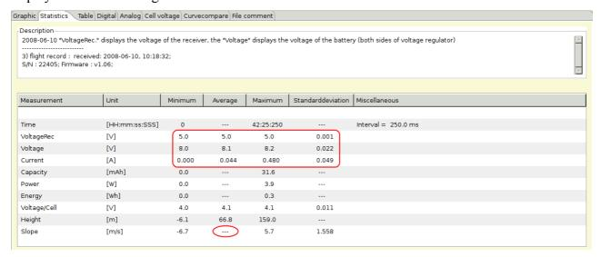
Below a motor measurement statistics view is displayed. All important calculation data and differences are red circled.
