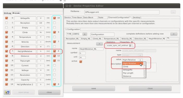
At the right hand side of the configuration panel are check boxes which enable a semi automatic scale synchronization. While checking measurement name will be compared to previous once and the fitting measurement ordinal will be added to the measurement configuration entry. Using scale synchronization will reduce the required space for scales and spend more for the graphics. Overlaying curves in this matter will allow direct comparison without using the curve compare window.
