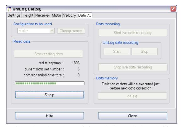
At the end of the read operation the data are displayed. The dialog gets back to its initial state. Only the progress bar is filled and the number of red data telegrams are displayed.
