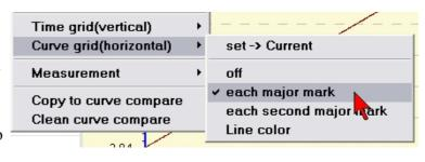
**Horizontal grid lines** are bound to only one measurement. The curve name used to adjust this will be displayed. Each second will only draw a grid line each second major scale mark.
