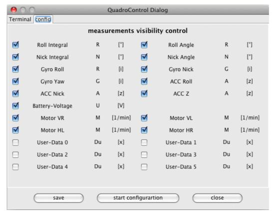
The displayed tabulator of the dialog is used to configure the visualization of the displayed data. Not checked curves get suppressed during visualization. Changes of this configuration can be saved and is used for all follow on visualizations.
