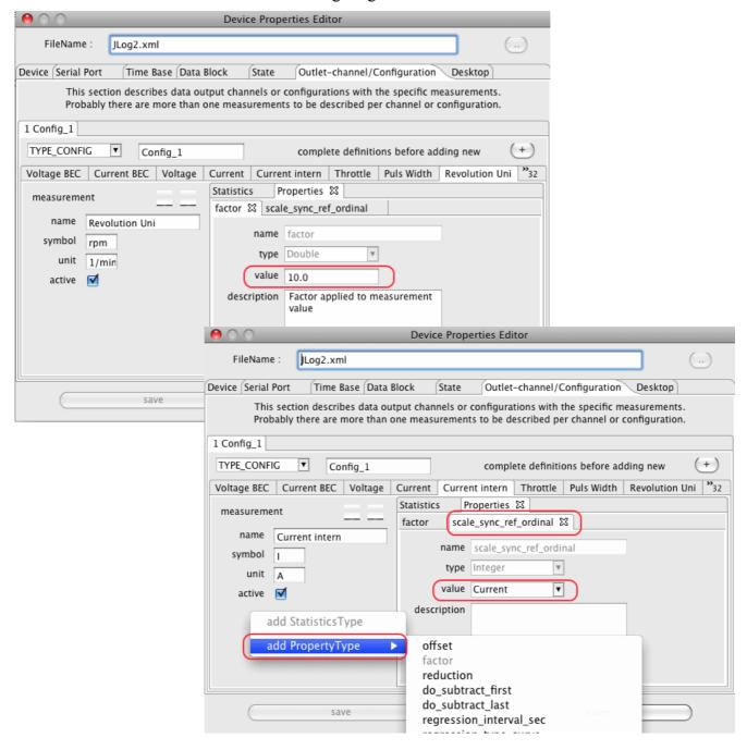
In cases where other sensors get connected it might be required to adapt a measurement factor or add an offset to adapt sensor capabilities to reality. All this can be done by using the DevicePropertiesEditor.
