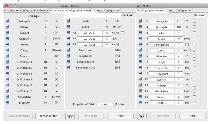
Entering the revolution were the Propeller drives 100 Watts, enable to calculate the Efficiency. Well, this calculation is not very accurate, but it helps for comparison.
