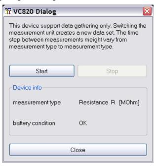
Switching the measurement unit or range at the multimeter itself will create a new data set. Pushing the "stop" button will stop gathering data.
