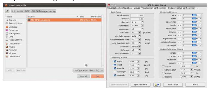
It is possible to configure a number of alarm thresholds and addresses to be used for Multiplex M-Link sensors.
