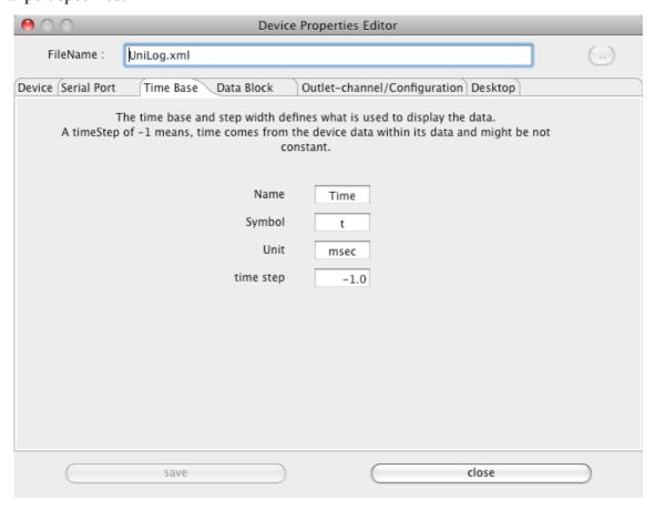
To configure the time base is simple. A value greater than 0 milli seconds as time step between the measurement points is voted as constant time gap. The time step value lower than 0 milli seconds signals that the device gives individual time steps. This must not mean that the time steps might not constant. The implementation for the particular device must handle this situation.
