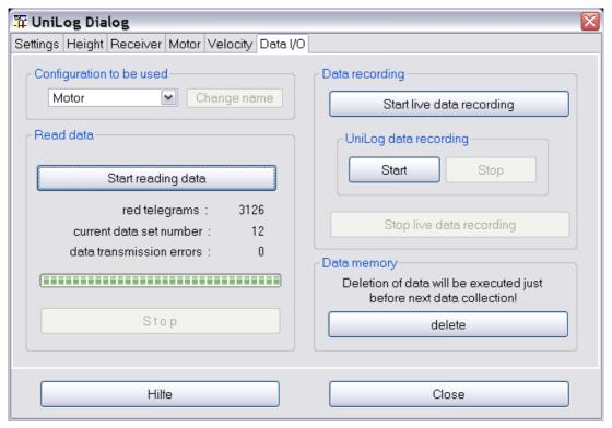
The Data I/O Tabulator enables to modify the configuration names. To change a configuration name it is required to push at first the button "Change name" to activate the change mode. After editing the name the operation is committed by the enter button. The new name will be displayed in the tabulator changed and will made persistent in the device configuration file.
